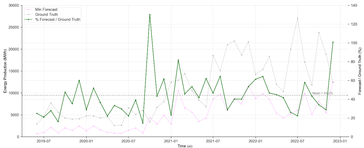
Figure 6: The comparison between the measurements at the Paradeisi substation and the minimum values of the monthly energy production forecasts from all ensemble members of the seasonal forecasting system, for the period from June 2019 to December 2022.
